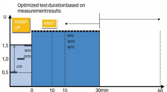
More information in less time: The cable condition is determined before the actual MWT - cable testing and dissipation factor measurement are combined. The subsequent MWT often takes less time than a normal cable test.
