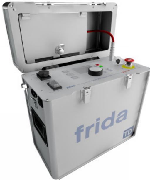
The Monitored Withstand Test (MWT) can be performed with the advanced, portable VLF testing devices from BAUR: viola TD and frida TD.
