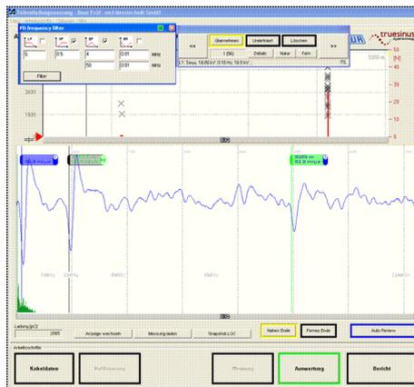
High-pass, low-pass and bandpass filters enable interference to be removed from the partial discharge measurement results display, which simplifies the analysis.
