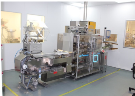
Blister machine in the production site of GE
