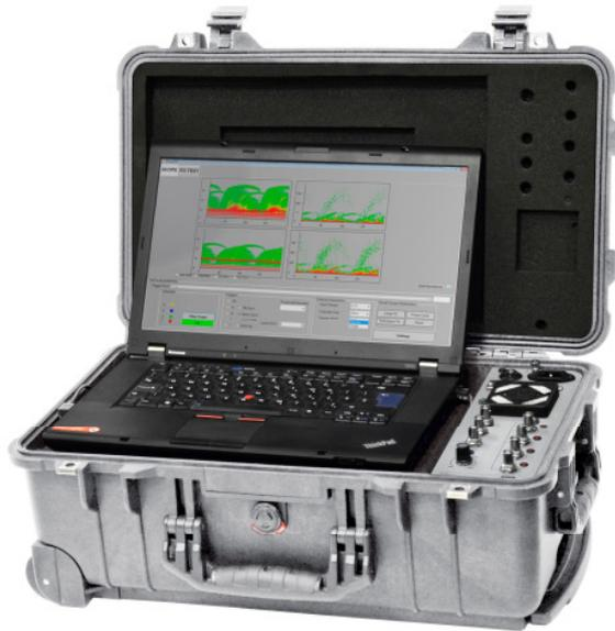
Quick tests for partial discharges in active power grids can be performed within minutes using the new portable measuring device liona from BAUR.
