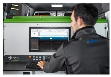
easily find their way around the interface and quickly obtain reliable results. However, the software also offers an expert mode in which experienced measurement engineers have direct control over processes and parameters. Help is also at hand for users whilst locating faults, with cable data and measured values linked to maps so that operators can quickly see where the problem lies.
