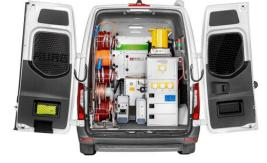
diagnostics. BAUR titron® – the future-proof all-in-one solution for cable fault location, cable testing and cable diagnostics.
