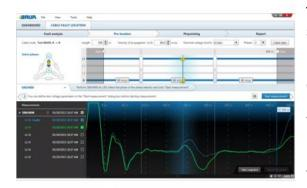
The Smart Cable Fault Location Guide speeds up cable fault pre-location and pin-pointing. The software can also be linked to the BAUR cable database and a geographical information system to narrow down the type and location of the fault even more rapidly. BAUR software helps during pin-pointing, too, and even protects the cable: The BAUR app shows the location of the fault on the display and allows the surge current generator to be
