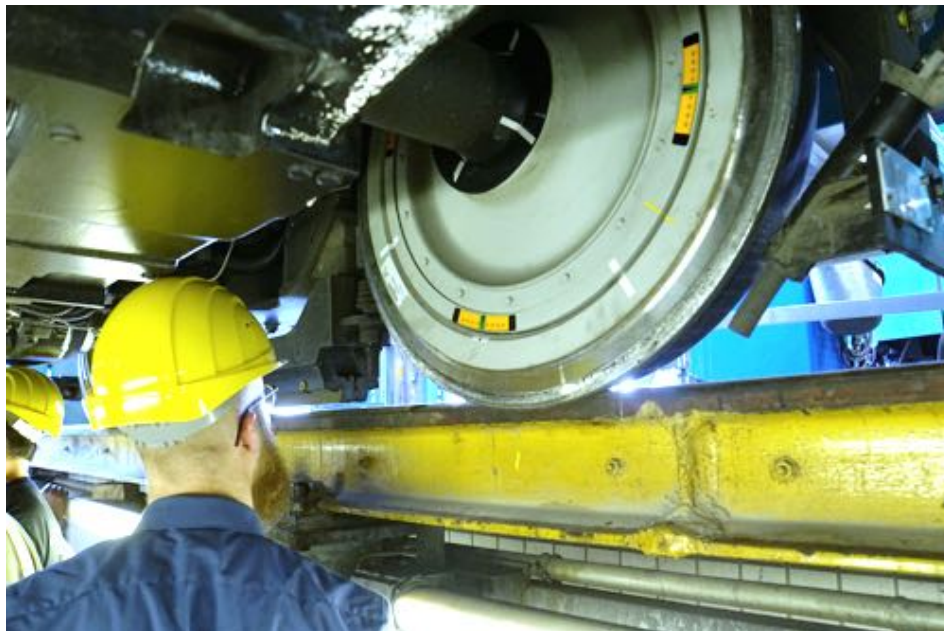
Aluminum instead of steel – The new BVV hybrid wheel BO 2000 achieves 50 kilogram in weight reductions. (Photo: Stadtwerke Verkehrsgesellschaft Frankfurt am Main mbH)
